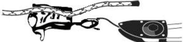
Position the clamp on the strand you are tensioning and attach the clamp to the "S" hook on the ratchet as shown.
